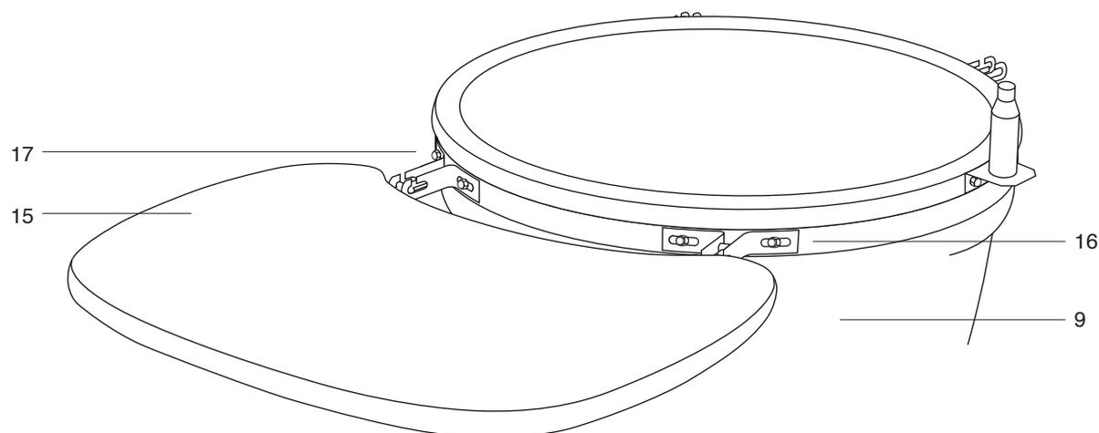
**STEP 16 -** Insert the 2x table hinge into each of the table brackets (16 & 17).
