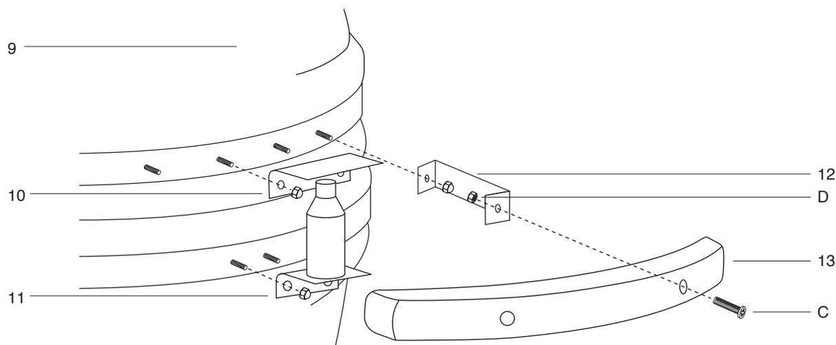
**STEP 10** - Attach the lid buffer top plate (10) to the lid of the Kamado Grill (9) by using the 2x pre-attached bolts and dome headed nuts.
