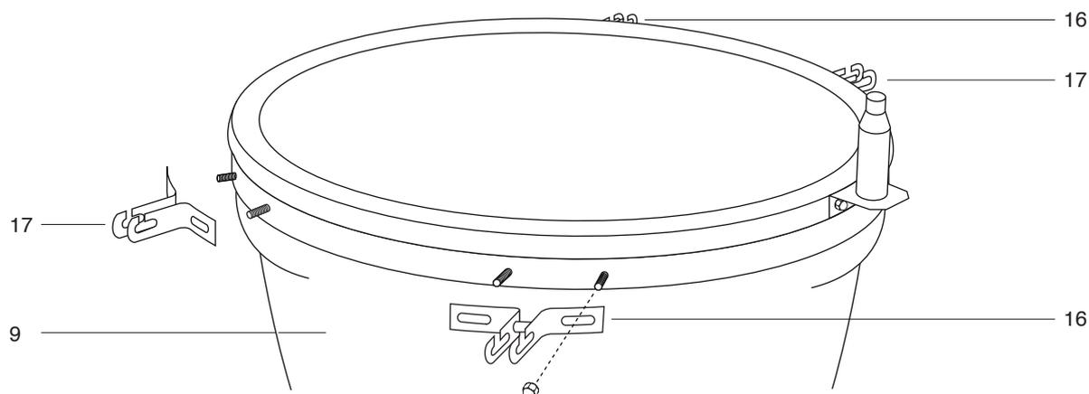
**STEP 14 –** Attach the 2x table brackets (16) to the Kamado Grill (9) using the 2x pre-attached bolts and dome headed nuts per bracket. Please note the position shown in the above diagram
