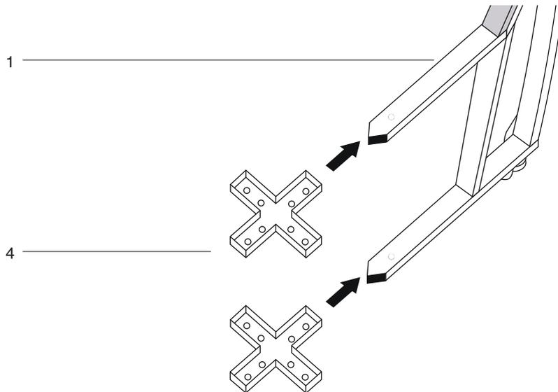
**STEP 2** - To assemble the cart insert the two cross pieces (4) into one of the four brackets (1) from both the top and bottom.
