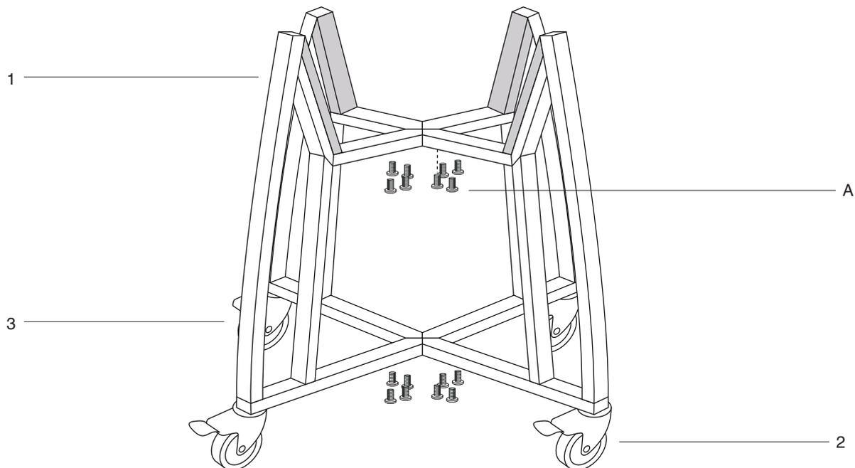
**STEP 4** - Secure the brackets (1) to the cross pieces (4) by using the 16x screws (A). Make sure the cart is secure and all of the screws are tight before placing the Kamado Grill (9) into it.
