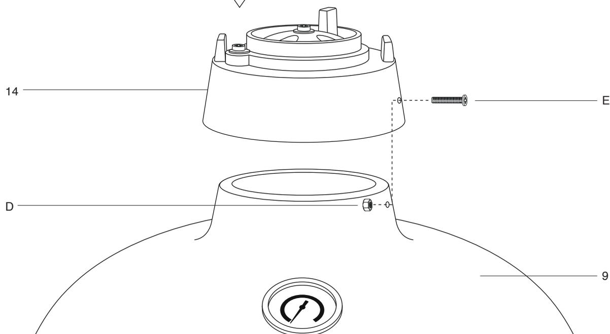
**STEP 13** - To attach the top vent (14) to the Kamado Grill (9) place it on top and align both the bolt holes. Secure using 2x bolts (E) and nuts (D) Ensure that the top vent bolt is on the left hand side when assembling it.
